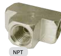
BQ265 NPT Tee Two 3/8-24 UNF ports One 1/8-27 NPT port
