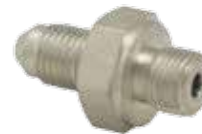
BQ157 -3 JIC to 1/8-28 BSPP 5/8" hex, 25.9mm overall length For use with bonded washer (dowty seal)
